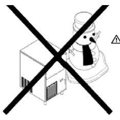
Location: The ice machine must be located inside temperature controlled room. Running the ice machine outdoors or in an area that the temperature can go outside of the working limits may harm the machine, and your warranty may become void. Ice machines are designed and built with the highest respect for security.
